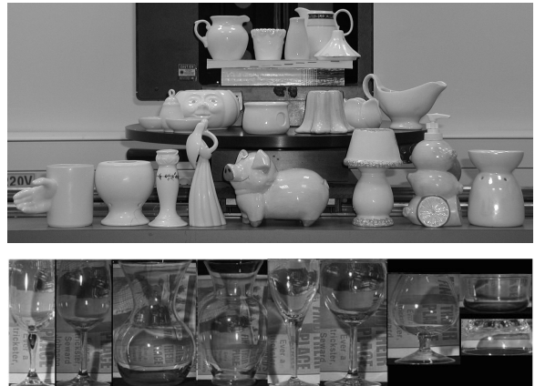
Figure 1: Objects tested in the experiments. Top – objects for Lambertian plus Specular test; bottom – transparent specular objects
